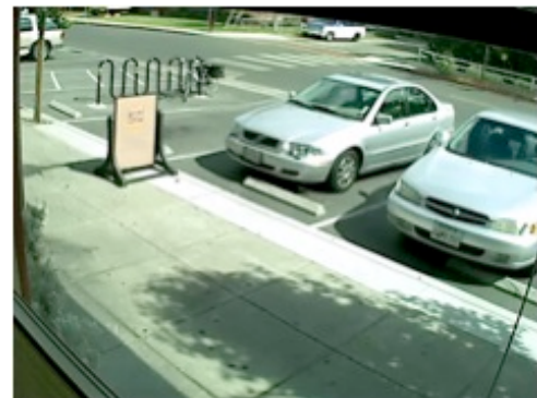
Motion detection can be triggered by light changes, reflections or swaying shadows.
